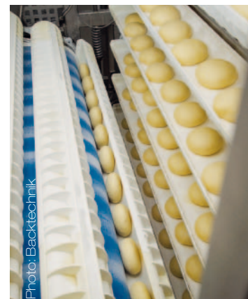
Left photo: The large kneading troughs provide sufficient space for the development of the individual dough pieces. Middle photo: Strong chains and several chain adjusters ensure operation runs very quietly and that wear and tear levels are low. Right photo: At the end of the stiffening zone the dough pieces are transferred from the proving trays to the discharge conveyor belt.
