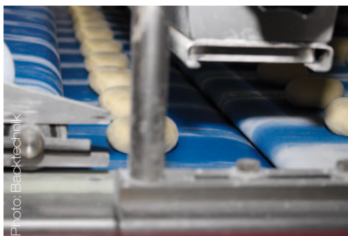
Left photo: To ensure the precise transfer of the dough pieces to the next station, the dough pieces are aligned on the belt. Middle photo: A pressing plate creates the correct form for the dough pieces before they are turned after about 20 minutes in the proving chamber. Right photo: A rapper on the potato powder container ensures the dough pieces are dusted promptly, consistently and finely.
