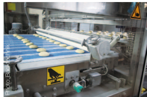
Left photo: The Softstar Plus dough dividing and rounding machine is suitable for doughs with a dough yield of 145 to 165. Middle photo: The robust link conveyors transport the 50 gramme dough pieces to the indexed and pivoting conveyor which doubles the number of dough pieces per row. Right photo: Very early on in the process the doughnuts are pressed into a typical doughnut shape.
