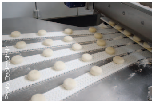
Left photo: The Softstar Plus dough dividing and rounding machine is suitable for doughs with a dough yield of 145 to 165. Middle photo: The robust link conveyors transport the 50 gramme dough pieces to the indexed and pivoting conveyor which doubles the number of dough pieces per row. Right photo: Very early on in the process the doughnuts are pressed into a typical doughnut shape.
