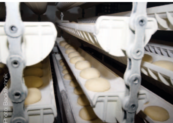
Left photo: The large kneading troughs provide sufficient space for the development of the individual dough pieces. Middle photo: Strong chains and several chain adjusters ensure operation runs very quietly and that wear and tear levels are low. Right photo: At the end of the stiffening zone the dough pieces are transferred from the proving trays to the discharge conveyor belt.
