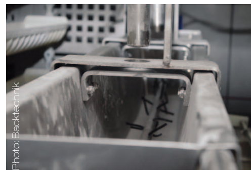
Left photo: To ensure the precise transfer of the dough pieces to the next station, the dough pieces are aligned on the belt. Middle photo: A pressing plate creates the correct form for the dough pieces before they are turned after about 20 minutes in the proving chamber. Right photo: A rapper on the potato powder container ensures the dough pieces are dusted promptly, consistently and finely.
