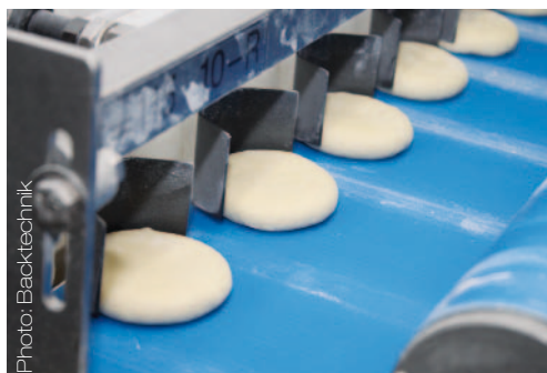
Left photo: To ensure the precise transfer of the dough pieces to the next station, the dough pieces are aligned on the belt. Middle photo: A pressing plate creates the correct form for the dough pieces before they are turned after about 20 minutes in the proving chamber. Right photo: A rapper on the potato powder container ensures the dough pieces are dusted promptly, consistently and finely.
