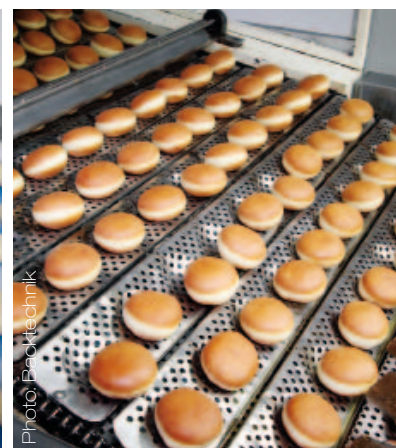
Left photo: The dough pieces pass through a lamella curtain out of the stiffening zone and are moved from the discharge belt to the baking tray. Right photo: The baked doughnuts can still drip a little before the relevant fillings are injected.
